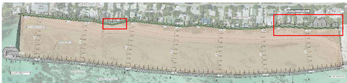
Figure 8: Overview of proposed reclaimed land with drainage on the land side (green) and potential land side infill areas highlighted (red bounded box)
